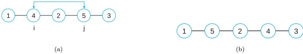
Figure 5: Route instance before (a) and after (b) the application of the swap operator.
