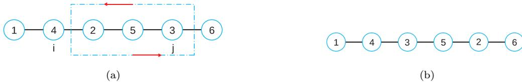
Figure 6: Route instance before (a) and after (b) the application of the 2-Opt operator.
