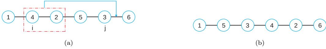
Figure 7: Route instance before (a) and after (b) the application of the Or-Opt operator
