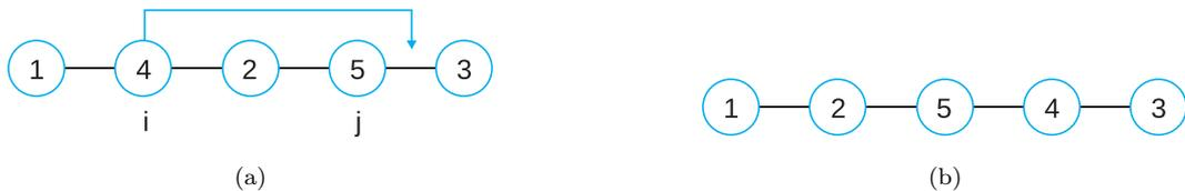
Figure 4: Route instance before (a) and after (b) the application of the Relocate operator
