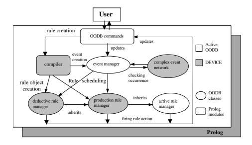
Figure 10. The architecture of the DEVICE system.
