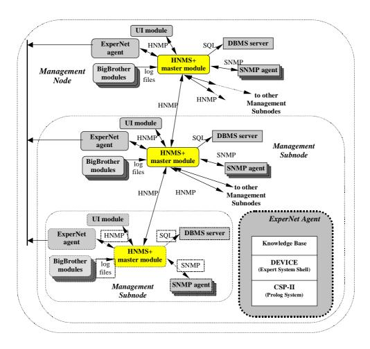
Figure 1. ExperNet system architecture.
